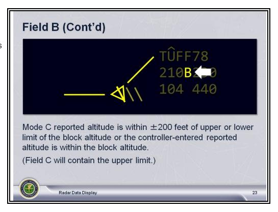
**NOTE:** An aircraft climbing or descending to a block altitude will display the highest altitude of the block when climbing and the lowest altitude of the block when descending, until the aircraft is in the block.
