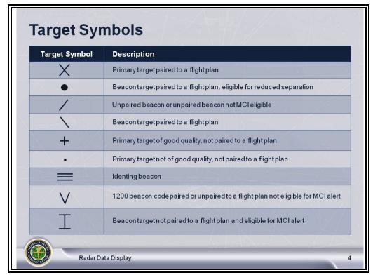
• Nine target symbols are used to display radar data.
